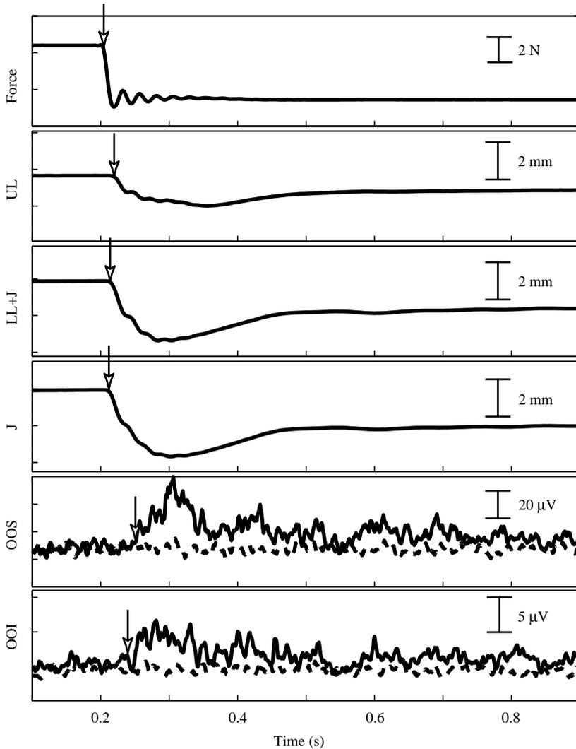
**Figure 2.** Perturbed responses of force, upper lip (UL), lower lip+jaw (LL+J), jaw (J), and EMG of OOS and OOI during a sustained production / $\Phi$ / (Subject A). EMG was rectified and smoothed with 5 ms temporal averaging. The arrows indicate the onsets of responses to the perturbation detected by the method described in the text.
