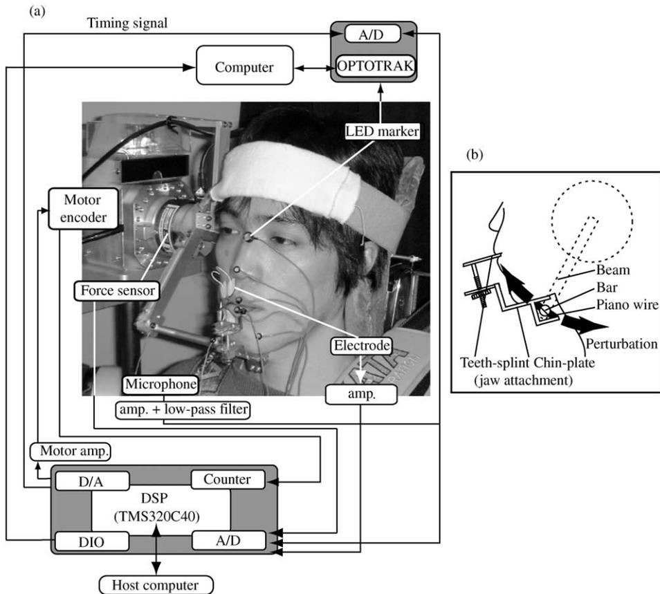
**Figure 1.** (a) Jaw perturbation system and experimental setup. (b) Side view of the configuration of experimental setup and the movement direction. A screw between a formed metal/plastic teeth-splint and a chin plate tightly fixes the jaw.
