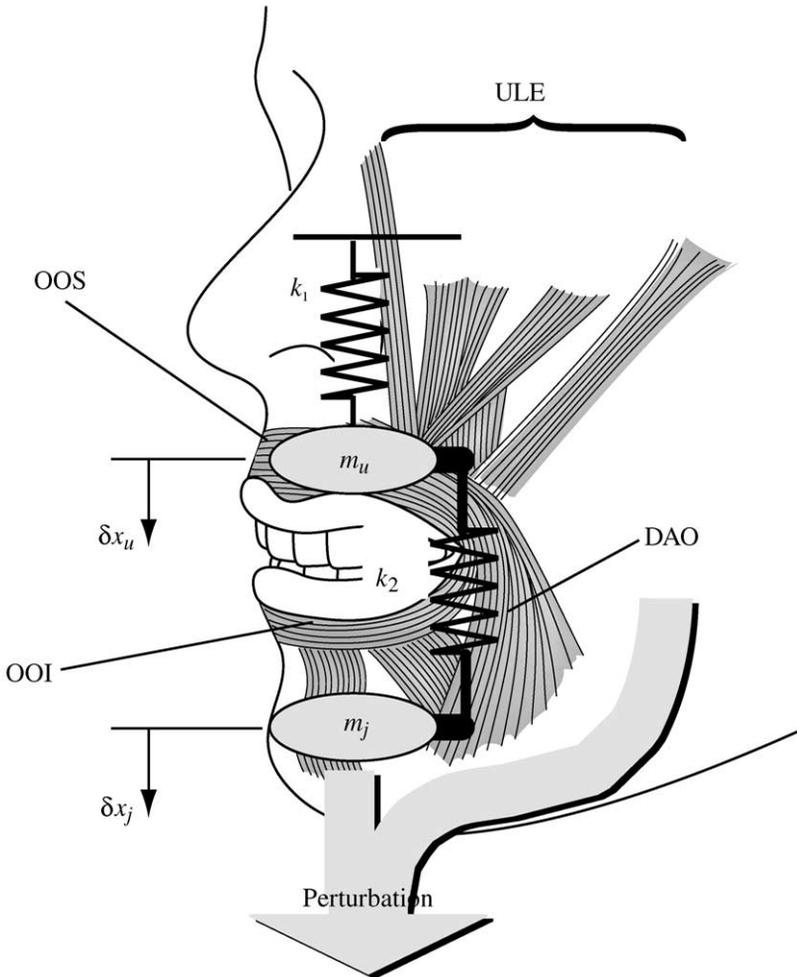
**Figure 7.** A serial connected spring model that represents the mechanical linkage of the perioral muscles and tissues between the upper lip and jaw. OOS, OOI, DAO, and ULE denote orbicularis oris superior, orbicularis oris inferior, depressor anguli oris, upper lip elevation muscles, respectively.
